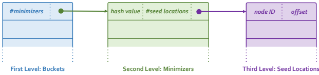
Figure 6: Memory layout of the hash-table-based index.
